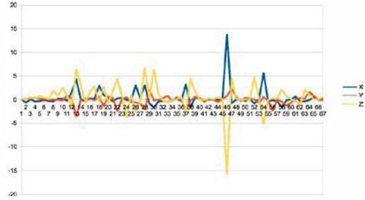
Fig. 8. Accelerometer values over time for swing of the tablet, as obtained from the tablet.
