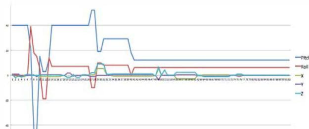
Fig. 11. Accelerometer values during a swing of the tablet, processed at the server to calculate the ball motion, once a threshold value of change is reached.
