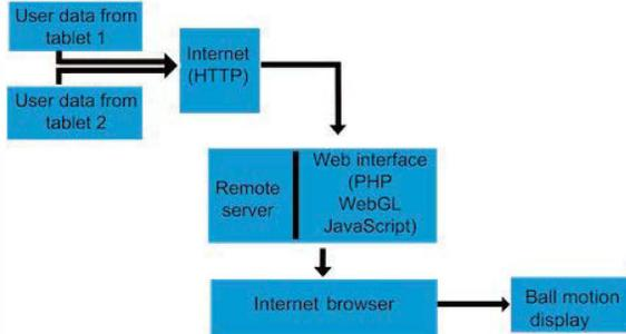
**Fig. 4.** Back-end system architecture of the TINB system. Data is filtered locally and transmitted to a remote server where calculations of the ball motion are carried out.
