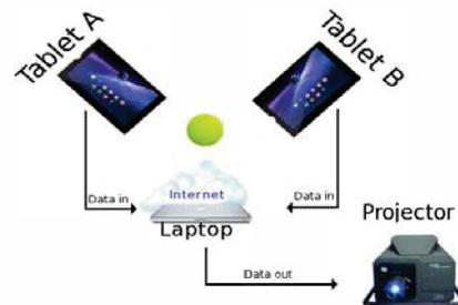
**Fig. 1.** Front-end system architecture of the TINB system. Two players play a game of paddle board with respective tablets. The data is relayed between the tablets and a third device, which can be connected to a projector to project the ball motion.
